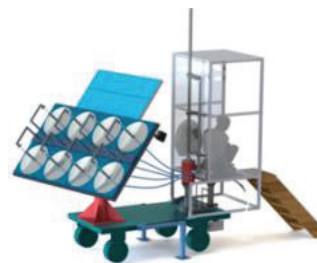
The portable SolChar includes the solar collector array connected to a bundle of Acrofusion™ cables to transfer heat energy.
